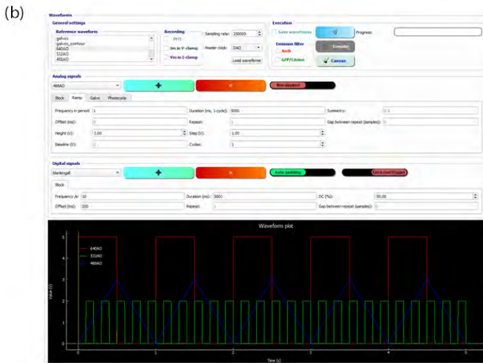
Figure 3.15: Class diagram and GUI of the waveform widget. The waveform widget takes charge of everything related to the DAQ system. Each waveform is received by a device's destination port, and its DAQ channel names are assigned in the lookup table file. The configured waveforms are displayed in different colours at the bottom.
