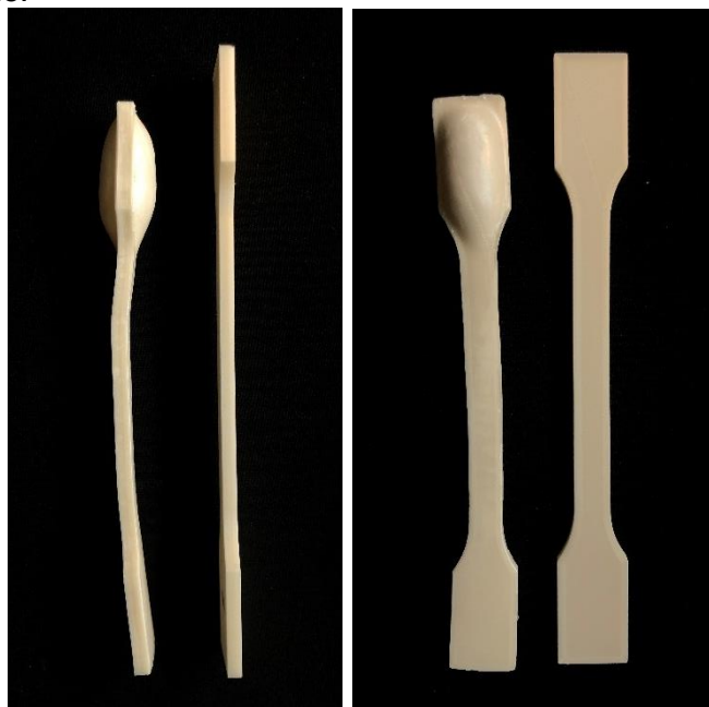
Figure 14. ISO 527 – The effect of the sterilization process on PLA specimens with 60% infill printed in the 0 degrees orientation. The specimen on the left is the sterilized sample in both pictures. The sample on the right is the unsterilized variant.
