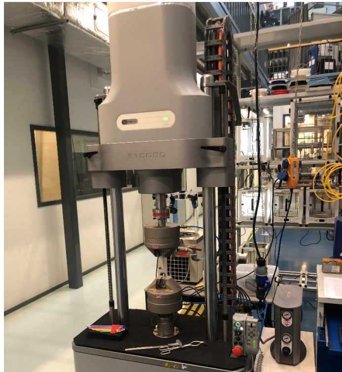
Figure 8. Instron Electroplus E10000 machine adjusted for ISO 527 tensile testing of 3D printed specimens.
