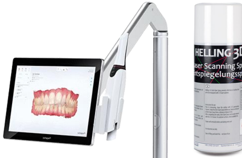
Figure 19. Left: 3Shape Trios Intraoral Scanner. The scanner can be seen in the holder next to the touchscreen. Right: Helling 3D scanning spray that was used for the small crevices in the 3D printed model.
