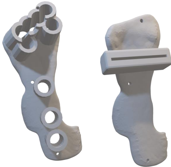
Figure 26. 3D models of a surgical drill guide on the left and a surgical cutting guide on the right. Both models were printed in BioMed Clear resin and in Polyamide 12 for dimensional tests. When opened in Word, models can be visualized in 3D.
