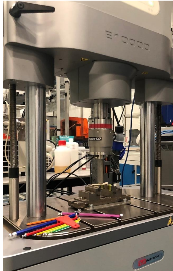
Figure 6. Instron Electropuls machine for mechanical tests. In this picture the machine is setup for ISO 178 flexural tests.
