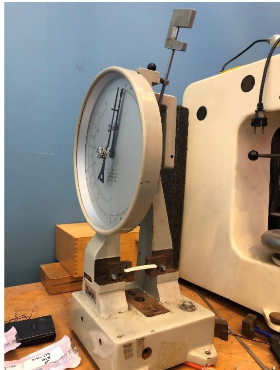
Figure 7. Charpy pendulum impact tester from Zwick Roell. The PLA specimen is placed in the middle on the supports and the pendulum is positioned at a 160 degrees relative to the point of impact.
