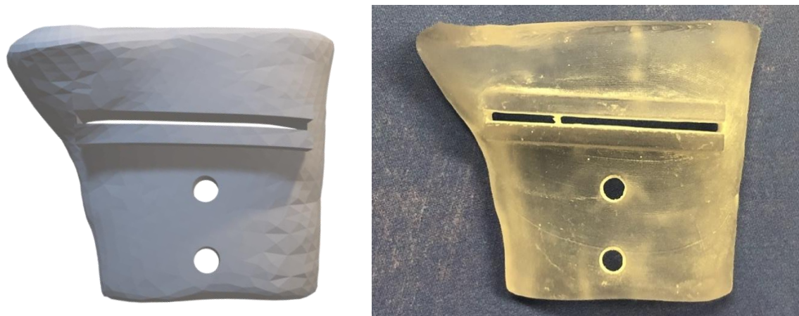
Figure 18. On the left: the digital 3D model of the surgical guide that is used for dimensional testing. When this thesis is opened in Word, one can view the model from different angles as it is implemented as a 3D model. On the right: 3D printed result in BioMed Clear resin.
