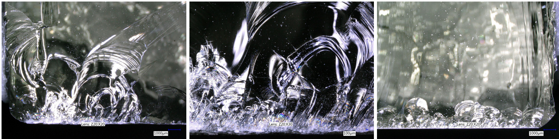
Figure III.31 - multiple failure origins in sample 2A left: failure original point at left corner middle: zoom of Left picture (note: different lighting) right: minor origins, non critical
