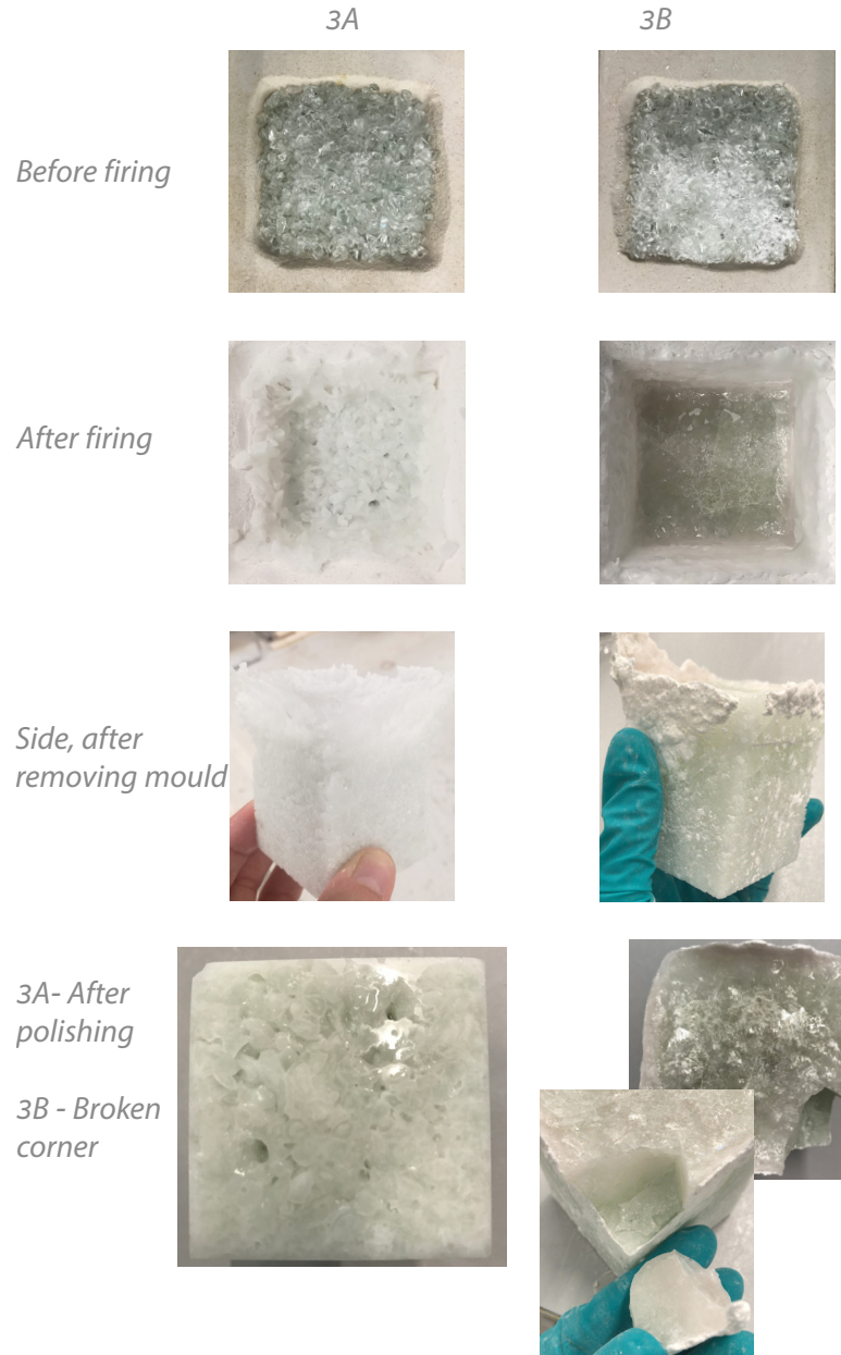
Figure B3 - melting experiment 3, top surface, at different stages with comment
