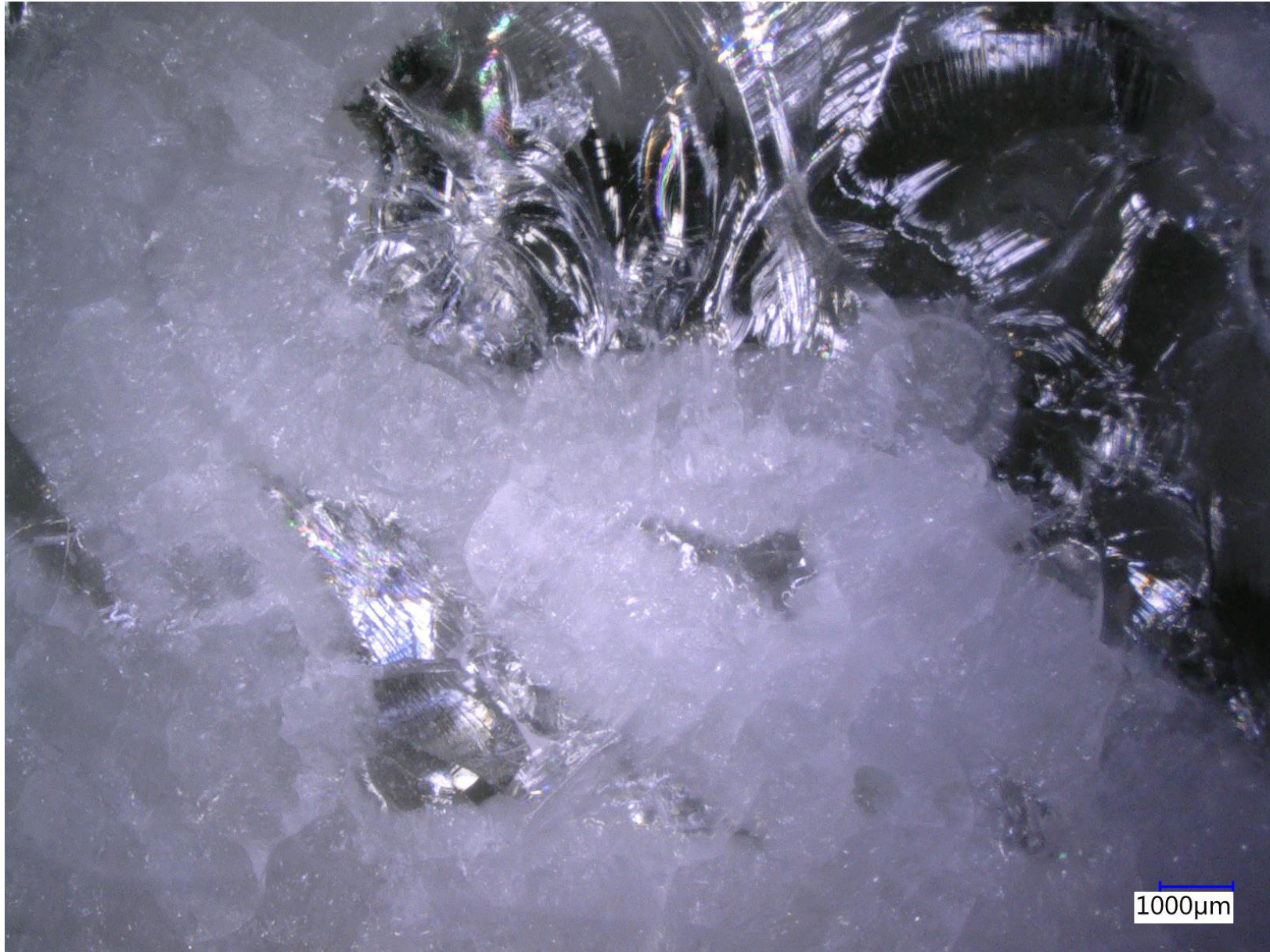
Figure F30 - sample 5A - Crystalline and glassy phase at the center
