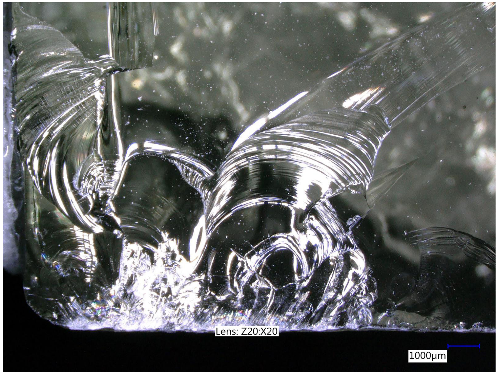
Figure F10 - sample 2A - Failure origin at bottom left corner
