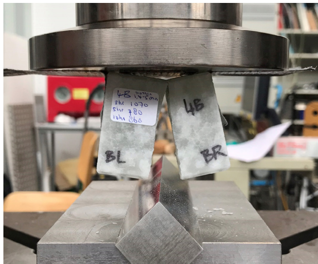
Figure D13 - sample 4B; left: set-up before and after splitting test. right: split surface
