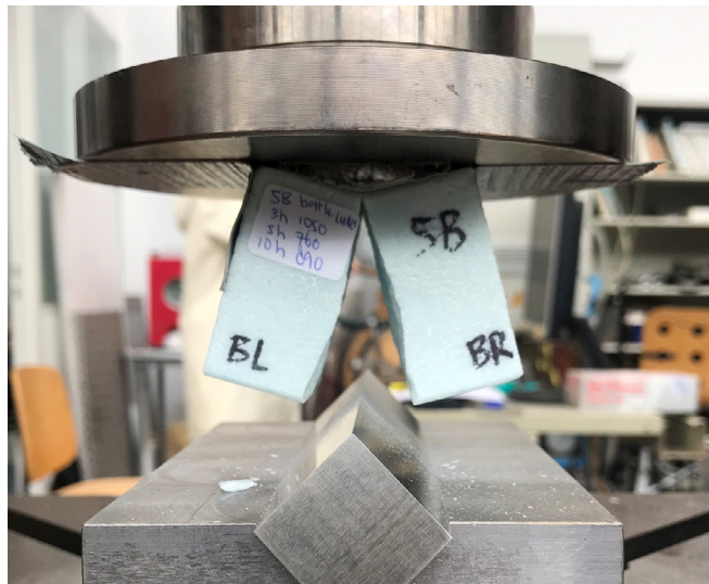
Figure D17 - sample 5B; left: set-up before and after splitting test. right: split surface
