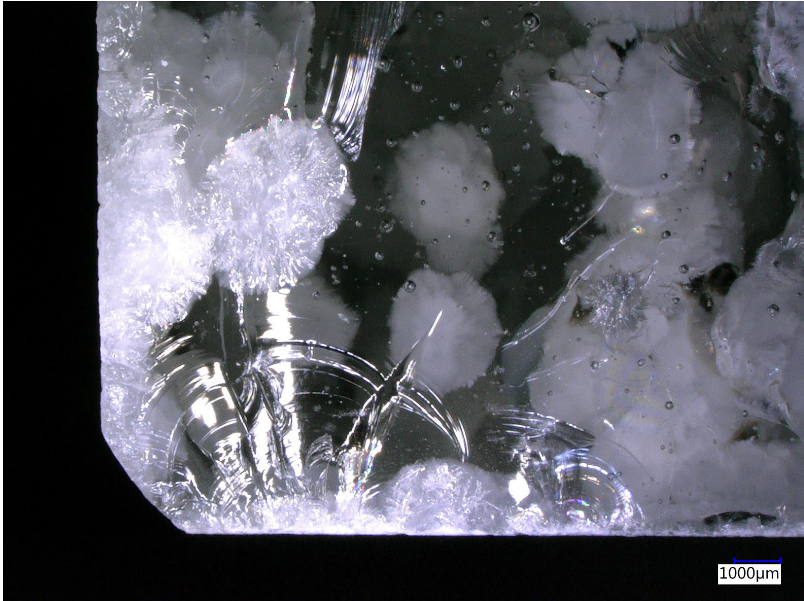
Figure F17 - sample 4B - Zoom of crack at bottom left corner
