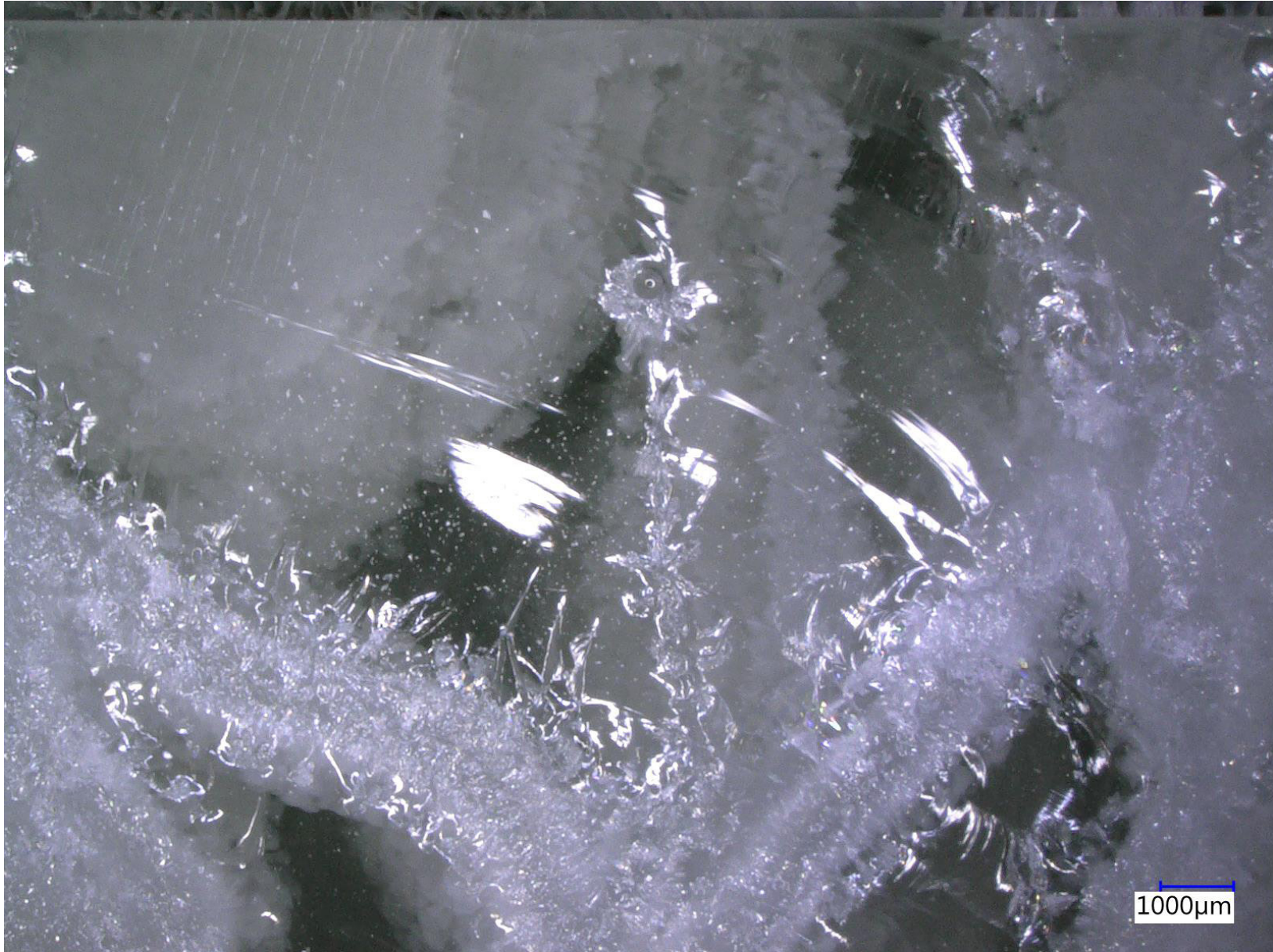
Figure F7 - sample 1B - Crack propagation from crystal to air bubble
