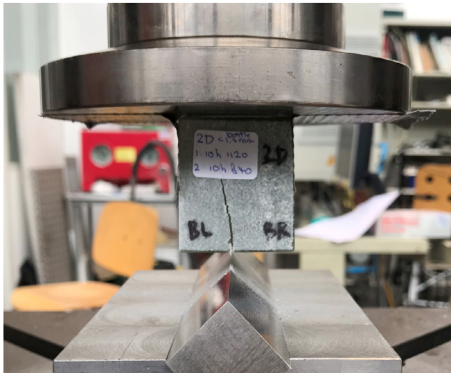
Figure D9 - sample 2D; left: set-up before and after splitting test. right: split surface
