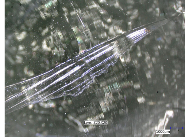
Figure III.32 - arrest line and crack propagation in sample 2A
