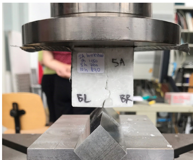
Figure D15 - sample 5A; left: set-up before and after splitting test. right: split surface
