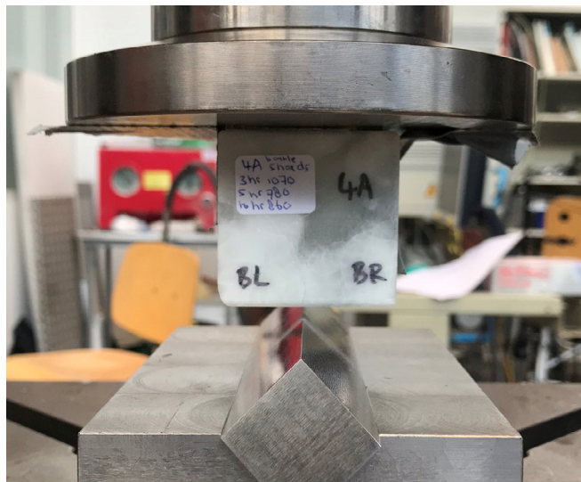
Figure D11 - sample 4A; left: set-up before and after splitting test
