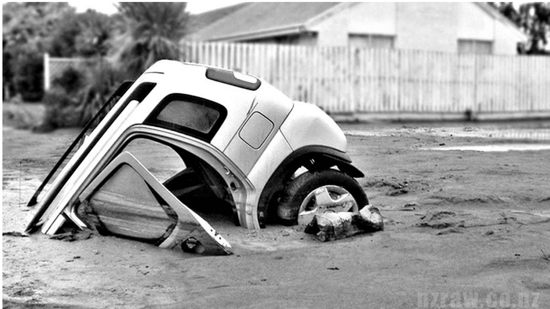
Figure 2.1: Sunken car stuck in densified soil after an liquefaction due to an earthquake.
