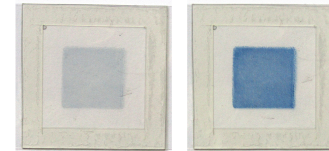
Figure 1.8: Switching between the bleached and colored state: Bleached state (a, b) and colored state (c, d).
