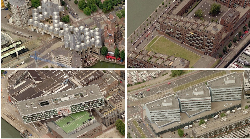
Figure 7.12: Examples of buildings in Rotterdam with an ambiguous notion of height. These cases illustrate that the ‘credibility’ of LOD1 models (extruding the building footprint to a single height) depends on the architecture of buildings. 24
