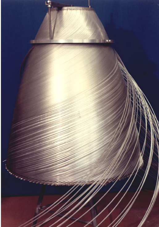
Figure 1.4: Tube nozzle, Arianespace [2]
