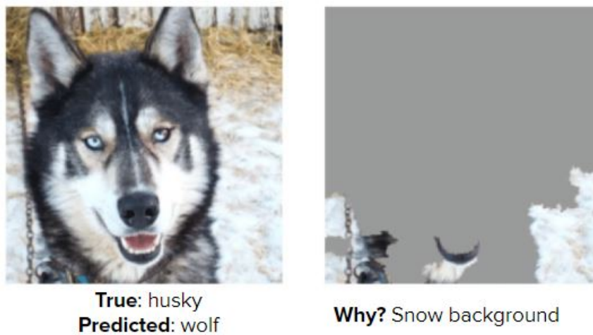
Figure 5.14: CV model bias - model predicts all images with snow backgrounds as a wolf
