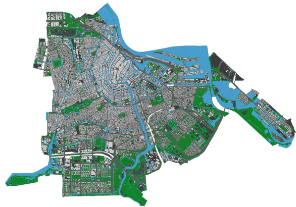
Figure 7. CityGML model of Amsterdam in LoD 1.
