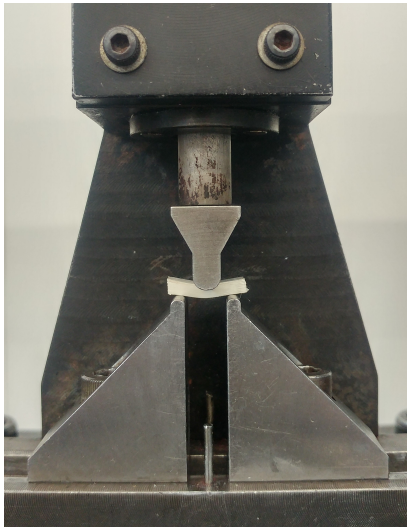
Figure 4.12 – Specimen in the 3-point bending fixture under test
