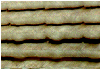
Figure C.5 – Close-up of Sample F80 0.35 090 2 showing an uneven layer profile but no interlayer feature.
