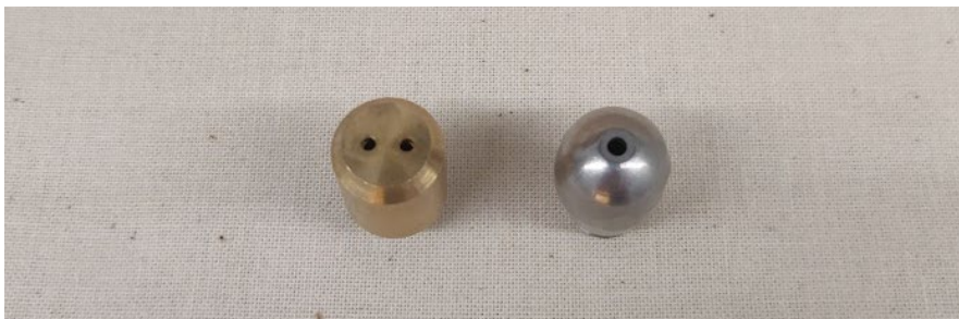
Figure 44: Comparison of vortex creation between nozzles with equal nozzle area, but different sized holes
