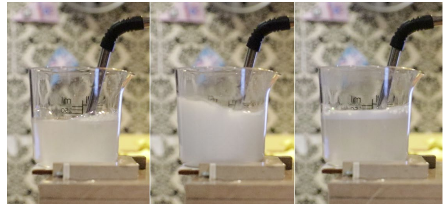
Figure 39: Turbulence induced by a single hole nozzle with diameter of 1.5mm of the thermocoil prototype.
