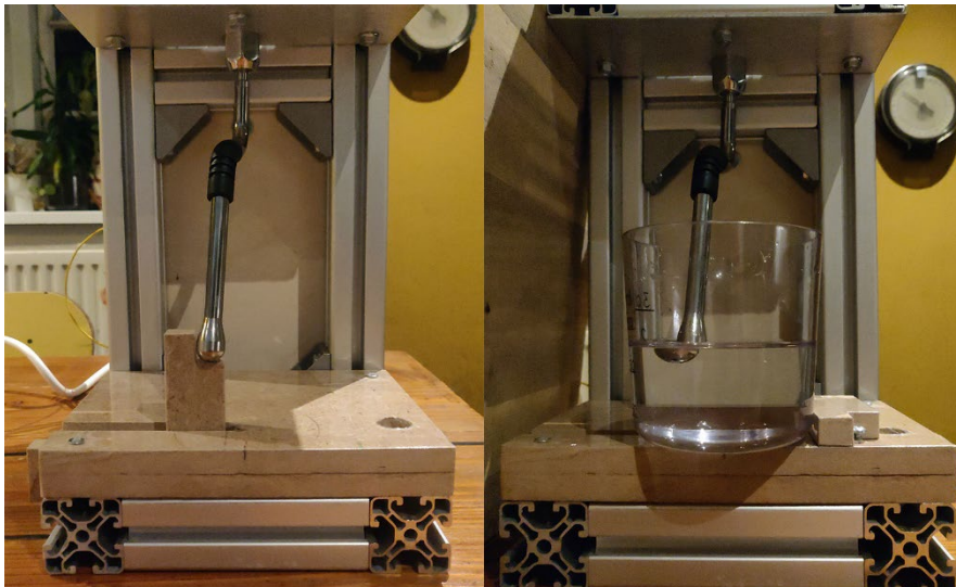
Figure 32: Consistent placement of steaming nozzle and dosing cup.
