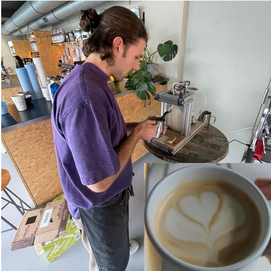
Figure 45: Testing of the development prototype with the final nozzle design being tested in situ, in the bottom right corner the milk foam quality is captured.
