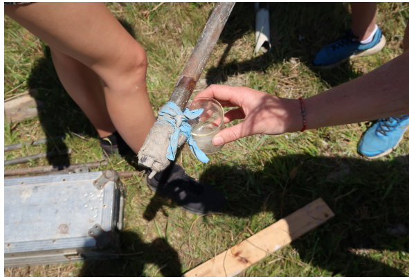
Figure C.4: Groundwater sampling using augur and syringe
