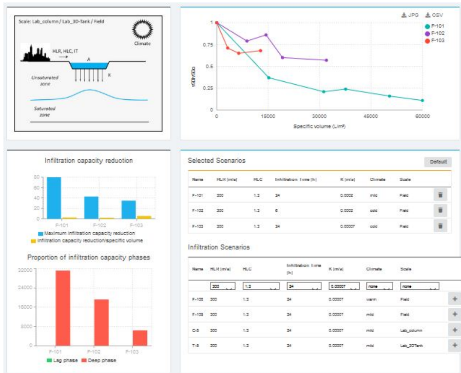
Figure G.1: Screenshot of the 'T01. SAT basin infiltration capacity reduction database'
