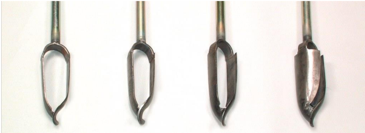
Figure B.3: Edelman drill bits for (from left to right): clay, combination, sand, coarse sand.
