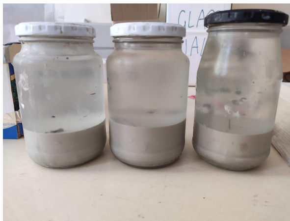
Figure C.5: The samples after sedimentation. The liquid phase was very clear, although the dirt on the jar and the condensation of the fridge doesn't imply this.
