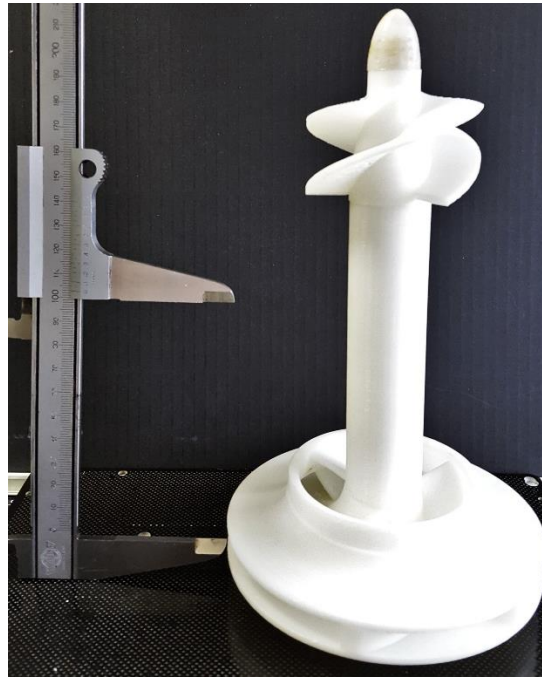
Figure 5.3: Optimized pump as reconstructed by 3D printing at the Osaka Institute of Technology.
