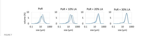
Particle size distributions as function of time. Full blue curve: after injection of algae; grey curve: 500 s after injection; dashed blue curve: before sampling for LabSFLOC2 measurements (when steady-state is reached).
