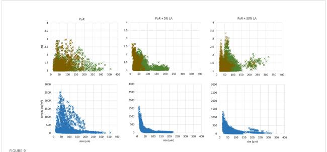
Top panel: Aspect Ratio (AR) as function of equivalent diameter. The brown color represents particles of effective density larger than 160 kg  $m^{-3}$  and the green colour particles of density lower than 160 kg  $m^{-3}$ . Bottom panel: absolute density as function of equivalent diameter. The data is obtained by LabSFLOC2 experiments.
