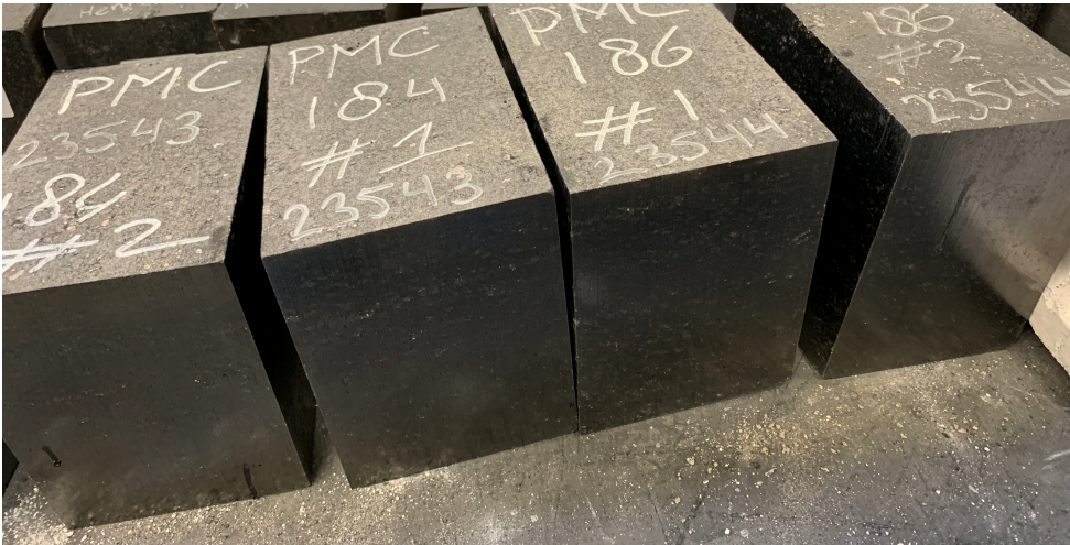
Figure A.4: Final bricks after pressing
