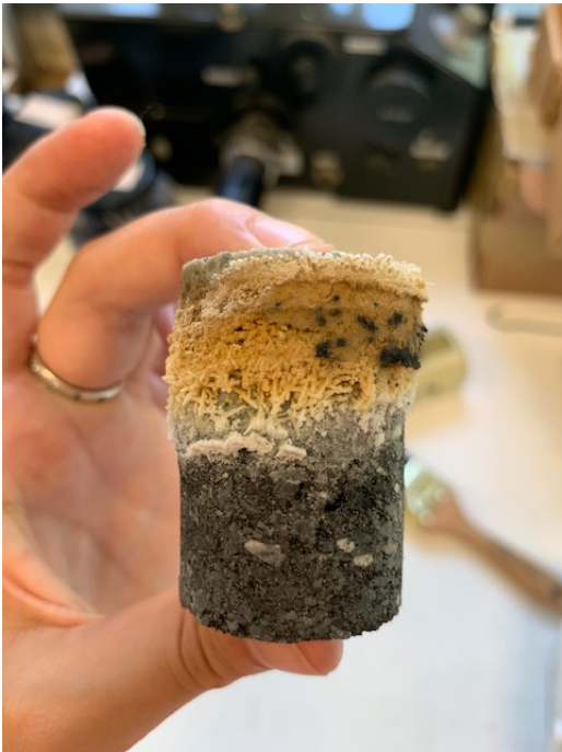
(a) PMC-2% binder sample after creep testing. Magnesium volatilised and deposited as magnesia "needles" on to the sample.
