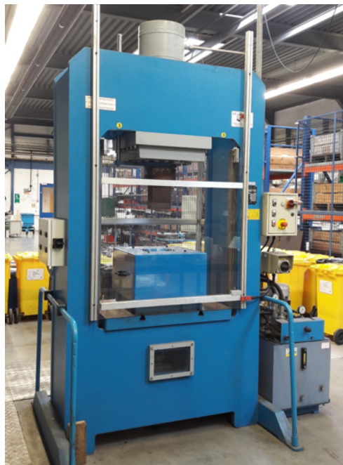
Figure A.3: Hydraulic press used to make the refractory bricks
