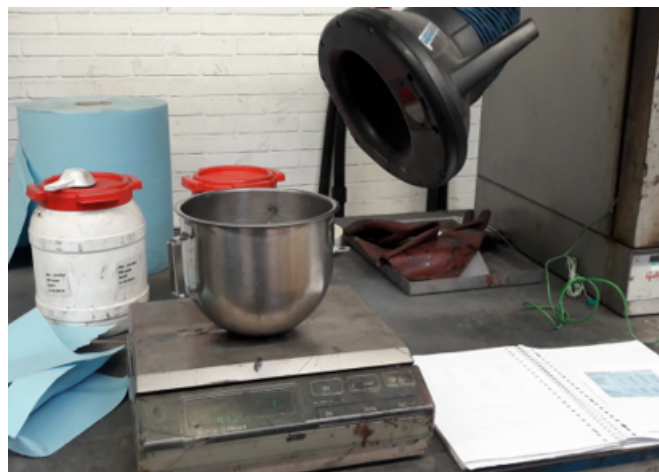
Figure A.1: Weighing the raw materials
