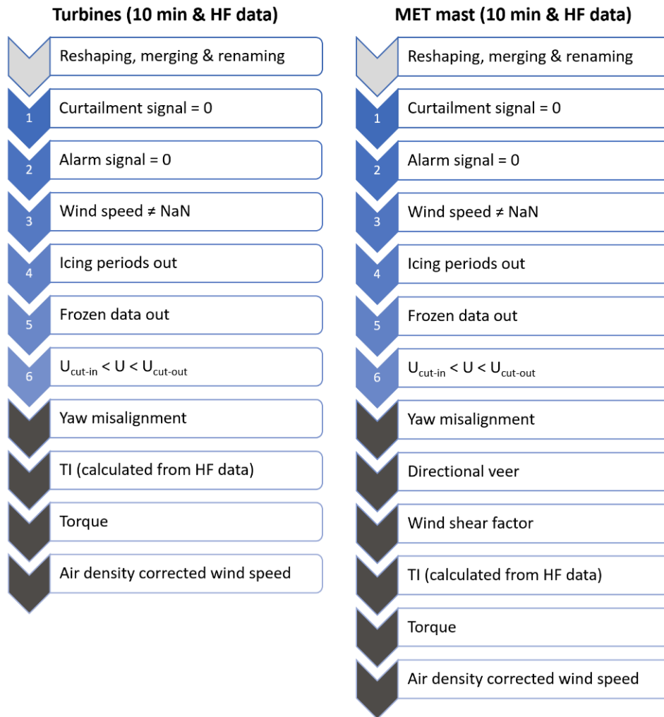
Figure 3.2: Filtering process for turbine data (left) and MET mast data (right)
