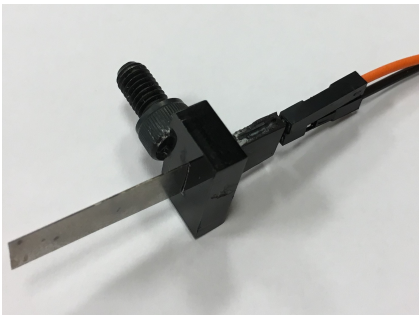
Figure C.1: Cantilever assembly of the LFRG prototype excluding proof mass.
