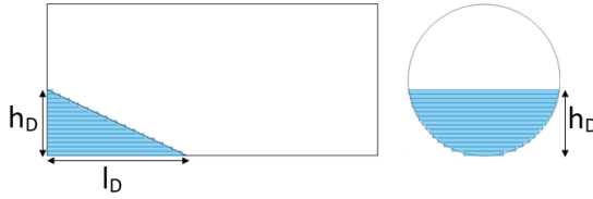
Figure 3.13: Rectangle approximation to compute MMOI of a partially filled, inclined cylinder of case D. Side view on the left, and front view on the right.
