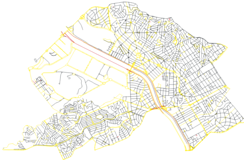
Figure 4.4: Road classification applied to the current road network. Black is mixed, yellow is separated and red is not suitable for cycling
