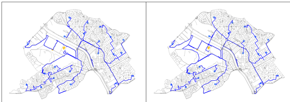
Figure 4.10: Minimum spanning tree (left: no cycling bridge; right: with a cycling bridge)
