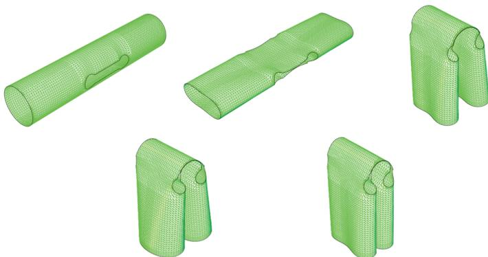
Figure 2.10: Working principle of tape spring. Retrieved from Mallikarachchi and Pellegrino (2010).
