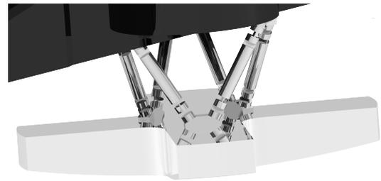
Figure 2.13: The secondary mirror interface. Adapted from Krikken (2018).
