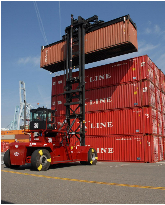
Figure 7.24: A toploader (source: www.taylormachineworks.com )
