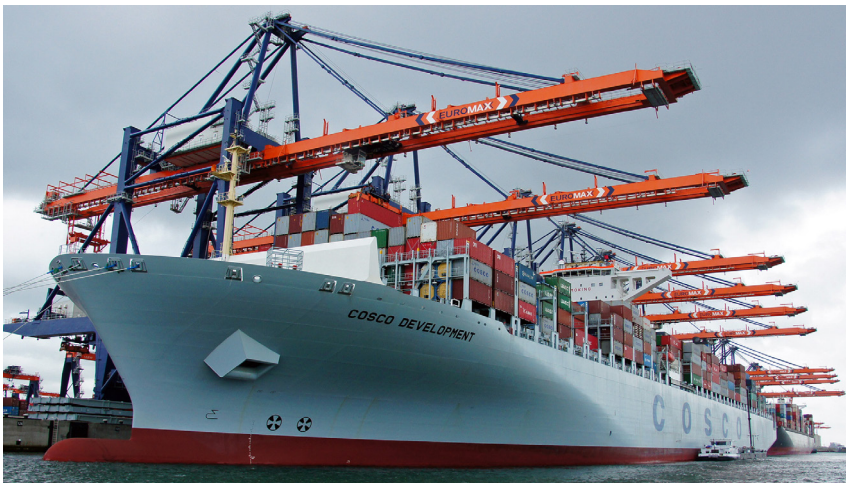
Figure 7.23: 13,000 TEU COSCO Development being handled by six STS cranes at Euromax terminal in Rotterdam (source: Kees Torn, Flickr, 11-09-2011)
