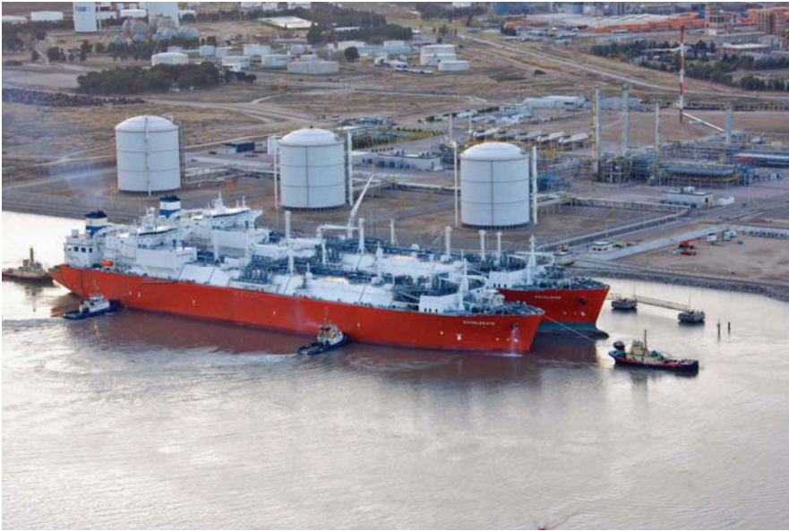
Figure 10.5 FSRU with shuttle carrier, Bahia Blanca, Argentina
