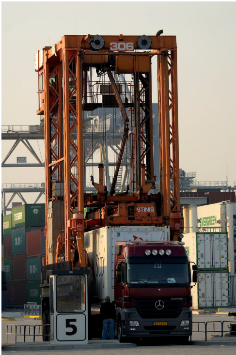
Figure 7.27: A straddle carrier (source: ECT)
