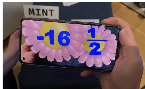
(a) The AR mobile prototype of “MINT Busters“ works with image tracking where the viewers interact with physical paper cards and the smartphone as an AR display.
