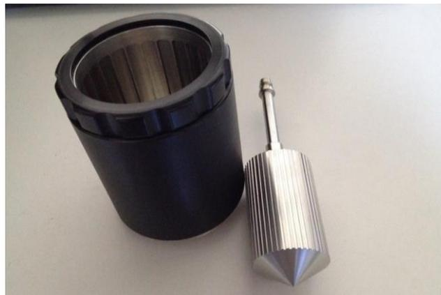
**Figure 3.2: Building Material Cell**
