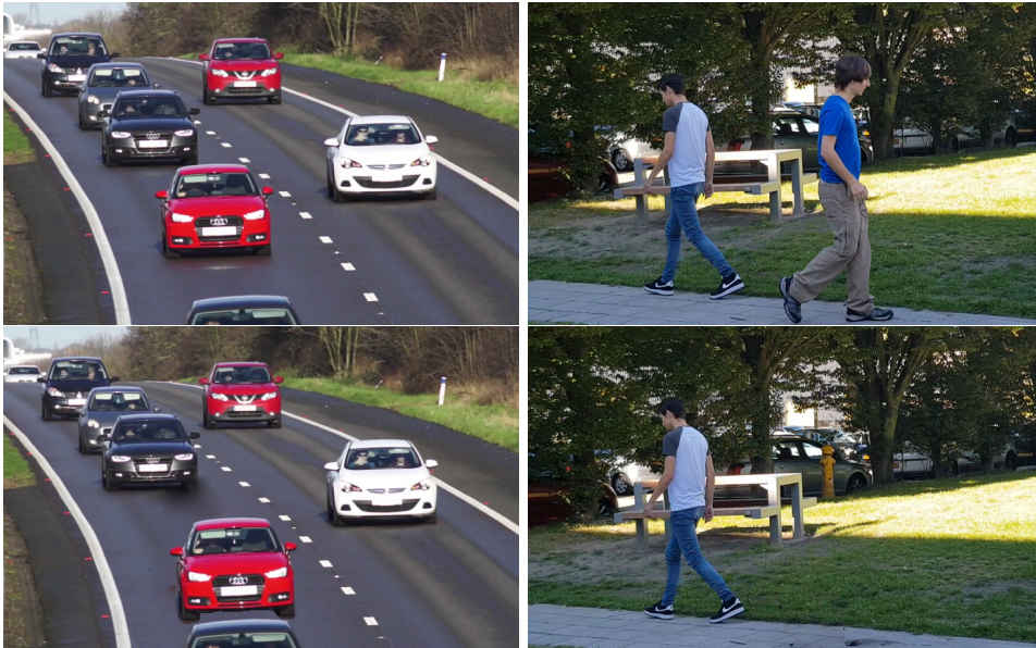
Figure 5.5: Temporally-driven hole filling. Top: original frames (cropped). Bottom: our approach recovers the background information for the disoccluded area when the red car is moved forward (left) and the person on the right is removed from the scene (right).
