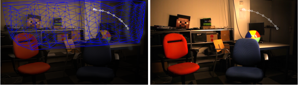
Figure 2.6: A Delaunay triangulation of light centers defines the weights to interpolate the captured light images.
