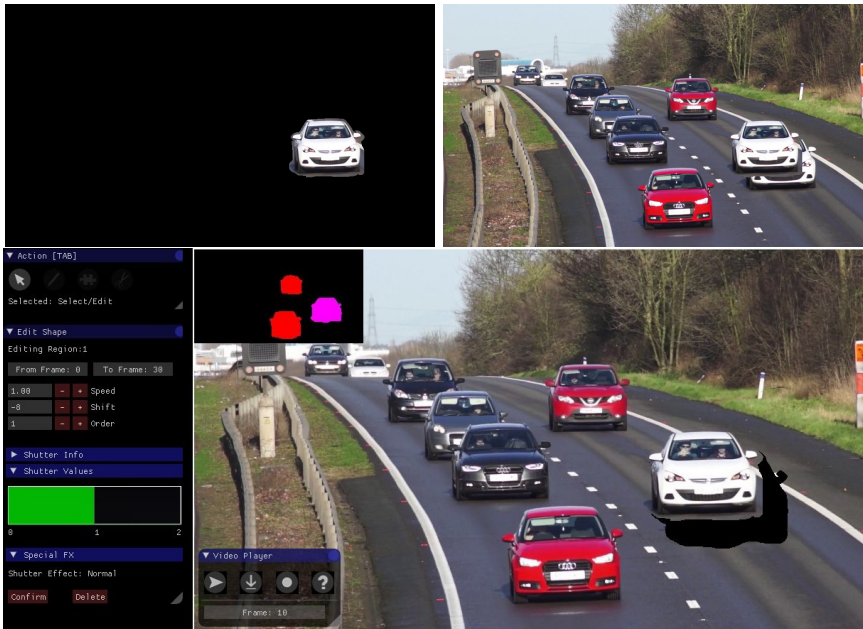
Figure 5.3: Compositing. Top: frame from the edited object video F_o (left). Direct fusion with the original sequence V creates a duplicate (right). Bottom: Real-time preview in our interface. The current instance is removed, and the black pixels on the removal region represent a mismatched region whose content must be reconstructed.
