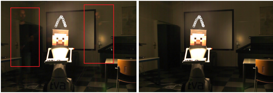
Figure 2.7: Ghosts by the light-handling person (left) are avoided by our approach (right).
