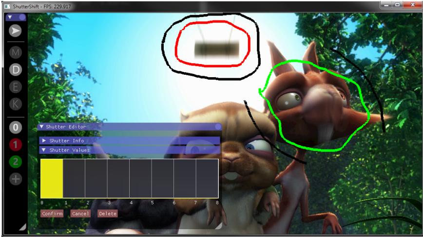
Figure 4.4: Interface for interactively defining shutter functions and their influence regions. Users design shutter functions using the bar graph editor, whilst additional details, such as the number of frames in the function, can be changed using one of the collapsed fold-outs. Influence regions are defined by drawing scribbles using the corresponding color. The results are immediately visible. The sequence is from the Big Buck Bunny movie by the Blender Institute [27].
