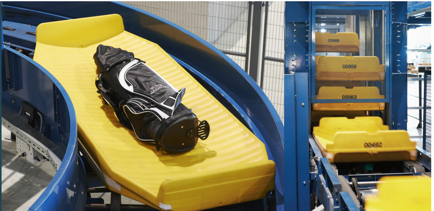
Figure 9: TUBTRAX conveying system (Source: Vanderlande)
