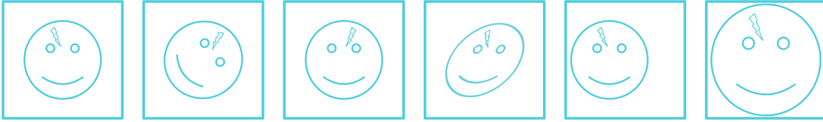
Figure 3.1: Examples of preprocessing operations. From left to right: the original image, a rotated image, a horizontally flipped image, a sheared image, a horizontally shifted image, and a zoomed image.
