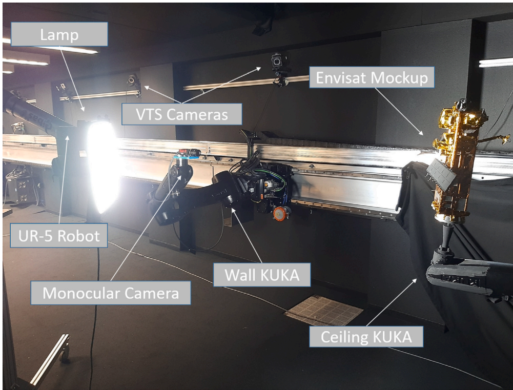
Fig. 3. GRALS testbed with the scaled 1:25 Envisat mockup mounted on the wall KUKA, the VTS and the monocular camera mounted on the ceiling KUKA. Two of the VTS cameras and the Sun lamp are also shown.
