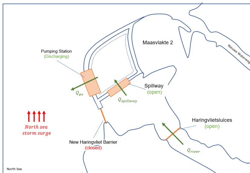
Figure 2.9: Operation of the Delta21 infrastructure during the combined occurrence of a storm surge on the North sea and a high river Rhine discharge. The New Haringvliet barrier will be closed to stop the storm surge, while the Haringvliet sluices and spillway are opened to allow for river water to flow into the Valmeer. The pumping station is used to simultaneously pump water out of the Valmeer.
