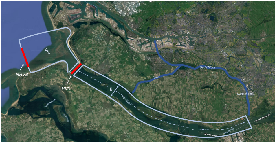
Figure 5.1: Domain for the hydrodynamic assessment of the barrier. With the tidal lake, located between the New Haringvliet barrier (NHVB) and the Haringvlietsluices (HVS). And the HV/HD channel that reaches from the HVS to the Dortsche Kill.
