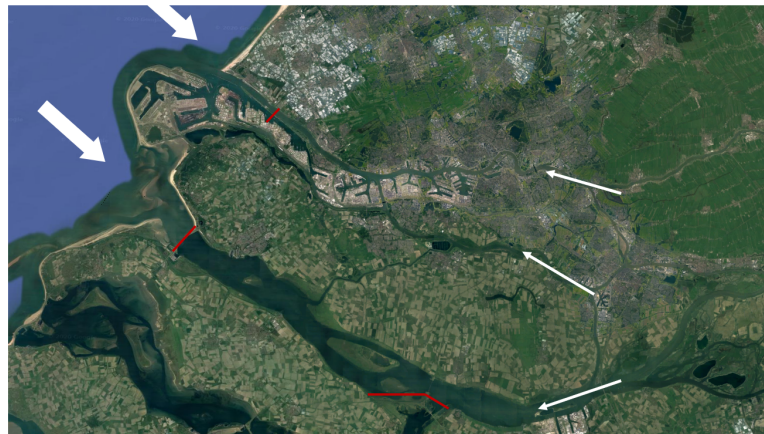
Figure 1.2: An overview for a possible critical flooding scenario for the RMD, during a long duration storm surge on the North sea, combined with a high fluvial discharge from the Rhine and the Meuse. In this situation, the barriers in the region (indicated in yellow) will be closed providing limited storage capacity in the Haringvliet estuary (source: Google Earth)
