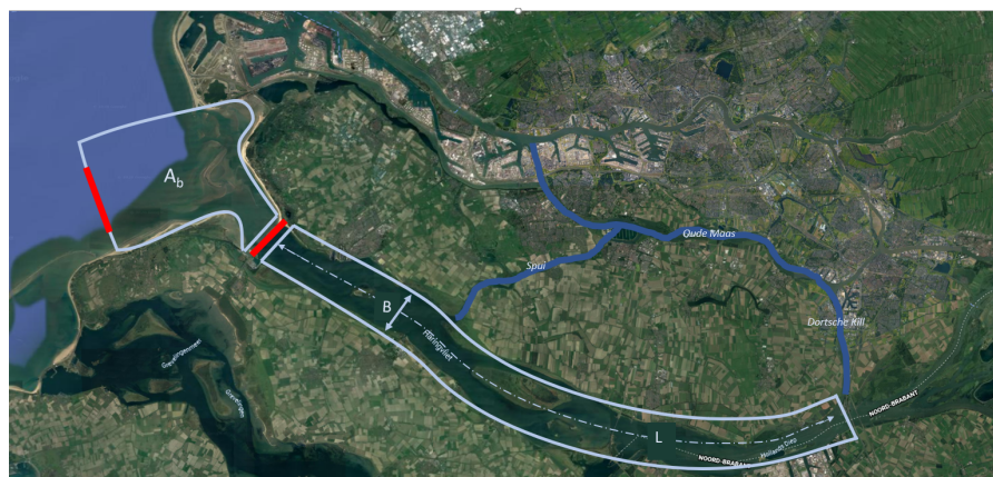
Figure C.1: Overview of the considered domain within the hydrodynamic assessment. The tidal lake is being considered as a short basin located in between the New Haringvliet barrier and the Haringvliet sluices, while the Haringvliet/Hollandsch diep is being considered as a canal reaching from the Haringvlietsluices to the Dortsche kill
