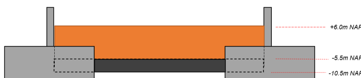
Figure F6: Alternate barrier layout, where the caissons are positioned higher relative to the other barrier elements
