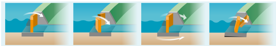
Figure 3.4: Failure mechanisms of water retaining systems from left to right: overtopping/overflow, failure to close, piping, structural failure.
