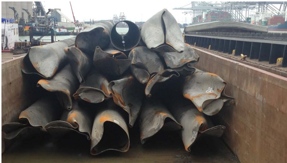
Figure 9: Heavily damaged pile toes
