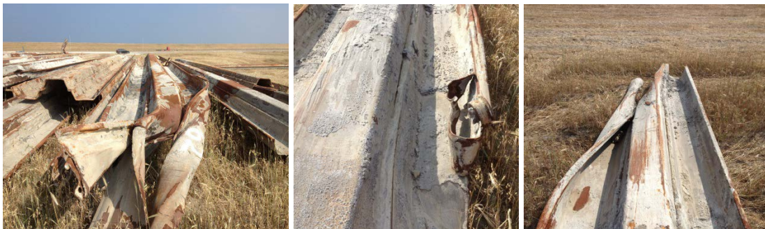
Figure 7: Sheet pile damages
