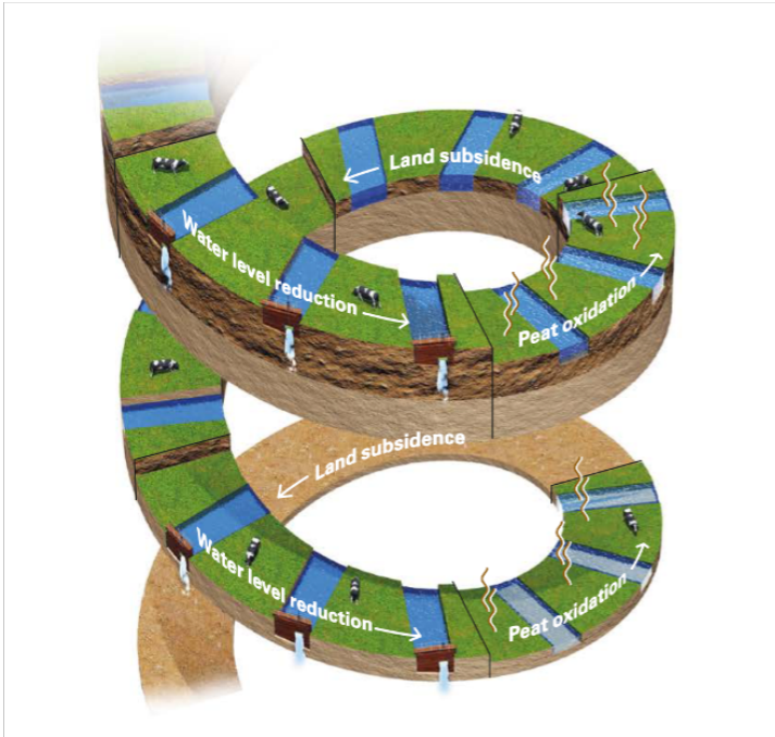
Figure 1.1: Visualization of the cycle of land subsidence caused by active water management in the Netherlands. Figure taken from the Netherlands Council for the Environment and Infrastructure (RLI), 2020.
