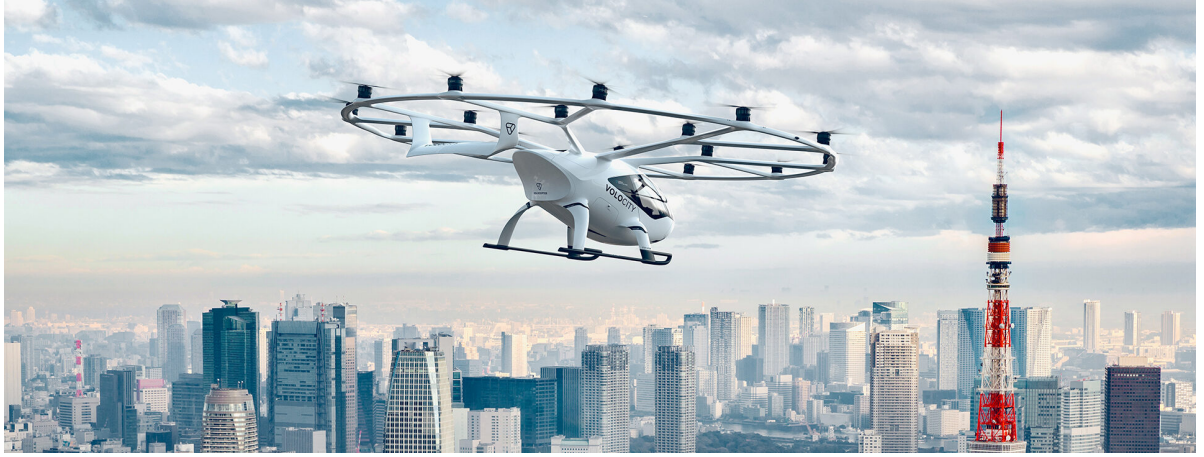
Figure 3.4: A multi rotor eVTOL aircraft concept designed by VOLOCOPTER flying over Tokyo [15].
