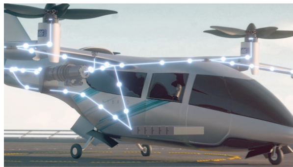
Figure 3.6: Rolls Royce hybrid eVTOL powered by its M250 turbo-generator [22].
