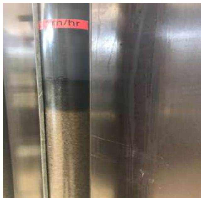
Figure 27: Sudden effect of addition of schmutzdecke
