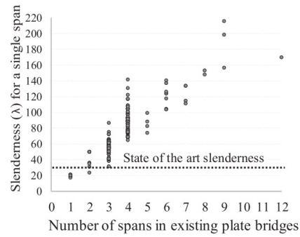
FIGURE 2.8: The span number in a plate bridge related to the required slenderness for a single span [Reitsema et al., 2015]
