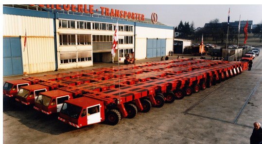
FIGURE 6.3: Self-Propelled Modular Transporter [Mammoet, nd]
