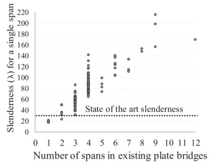
FIGURE 7.20: The span number in a plate bridge related to the required slenderness for a single span [Reitsema et al., 2015]
