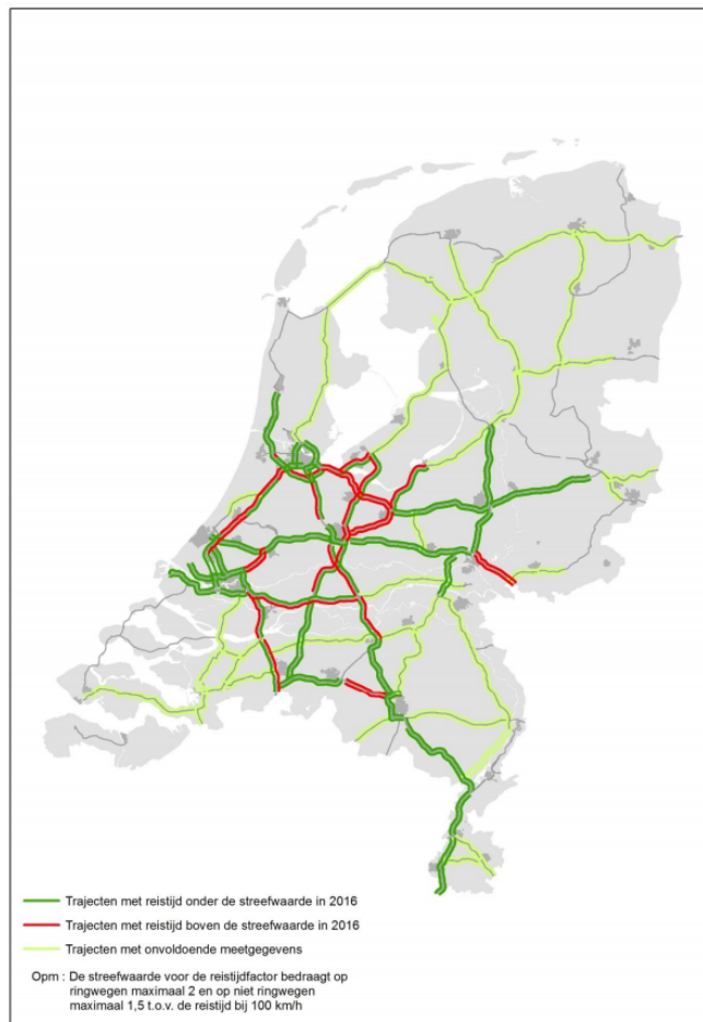
FIGURE 3.6: Overview of Dutch infrastructural network and the most heavily congested parts [Rijkswaterstaat, 2017]
