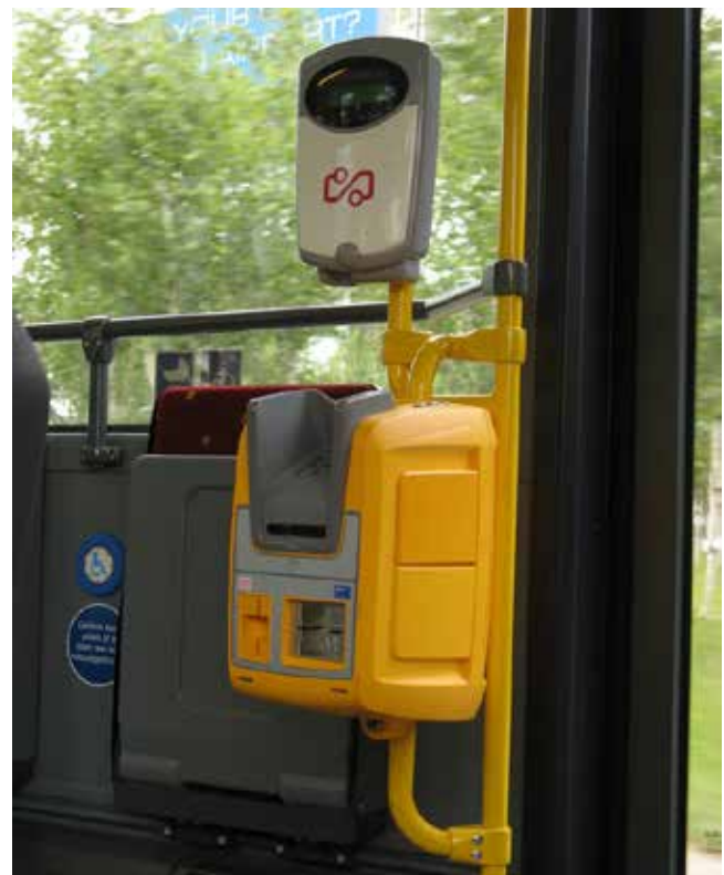
A Connexion onboard chipkaart fare reader with a debit card top-up machine underneath.
