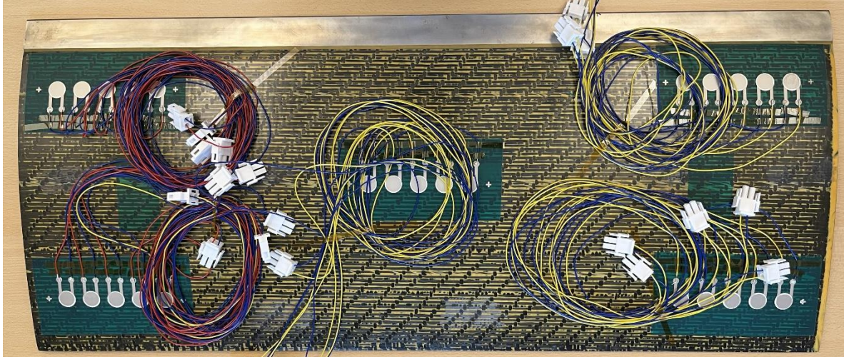
Fig. 1. Fully sensorized FOD panel with five printed sensors arrays plus connecting wires for data acquisition
