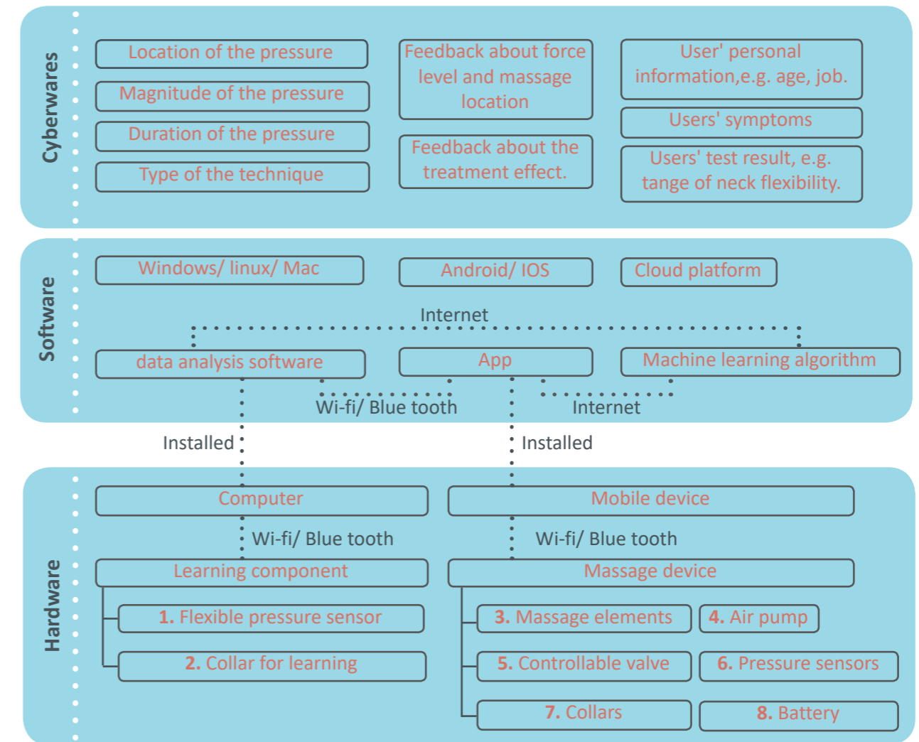
Figure 37: Layered model of the system
