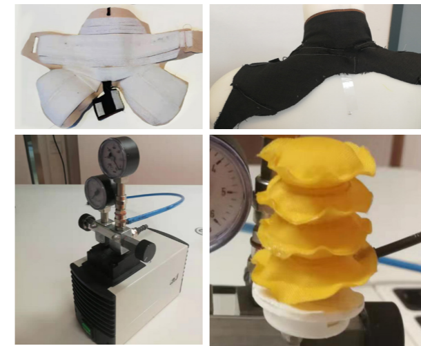
Figure 79: Prototype of massage actuator
