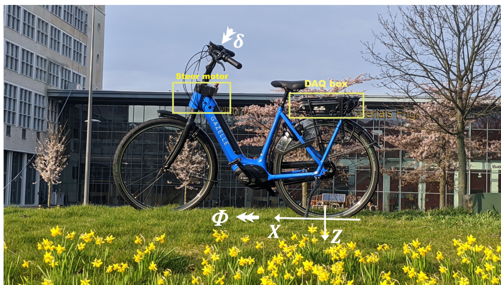
Figure 2 Second prototype balance assist bicycle at Delft University of Technology in collaboration with Royal Dutch Gazelle and Bosch eBike Systems. The steer motor and the data acquisition box (DAQ) are annotated in the image. The roll angle ( \phi ) around the X axis (forward) and the steering angle ( \delta ) around the steer axis are also shown.
