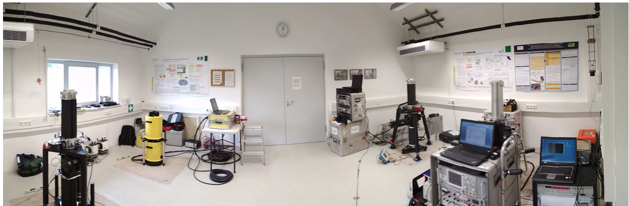
Figure 1. Sketch and Photo of the New Gravity Laboratory at Geodetic Observatory Wettzell on May 15, 2018. The pillar G is occupied by the SG030 and for AG measurements the central room is equipped with 4 pillars. The pillar H was not used during the comparison. The surface centre of each pillar is marked by a small brass benchmark, indicating the position A at each pillar.
