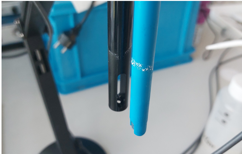
Figure 4.2: Photo of scaling on the EC and pH electrodes after 20 hours of reaction time.
