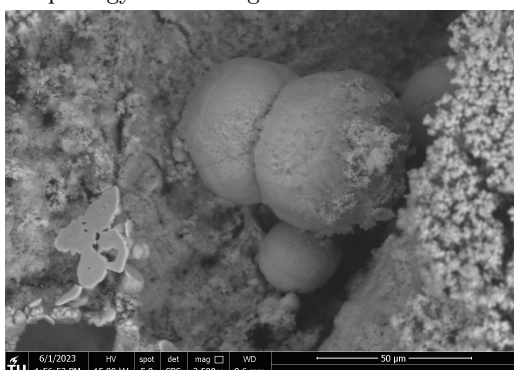
(c) Sample LY1 - 0.25 - 5 showing a spherical morphology at low magnification.
