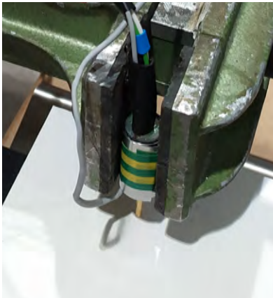
Figure 6.11: Force-stroke characteristic measurement setup for HTDA2.1 with backiron. The vice holds the device against a kitchen scale while also enabling us to adjust the distance between the device and the scale accurately.
