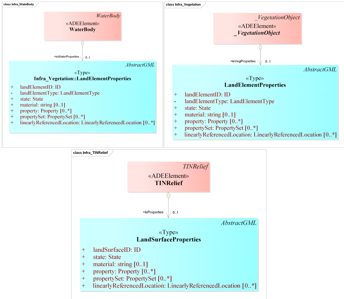
Figure A1. The UML excerpt depicts existing CityGML classes of CG::TINRelief , CG::WaterBody , CG::PlantCover , CG::SolitaryVegetationObject extended to include attributes from LandInfra LI::LandSurface , and LI::LandElement classes, respectively, in the CityGML Infra ADE.
