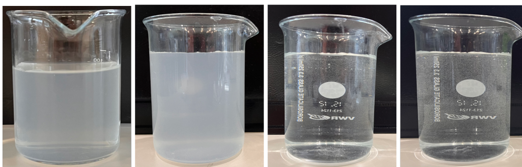
Figure F.2: 0.5 M solutions of the different \text{NH}_4\text{Cl} batches tested. From left to right: LabDiscounter (original), LabDiscounter (other batch), Thermo Scientific and Carl Roth.
