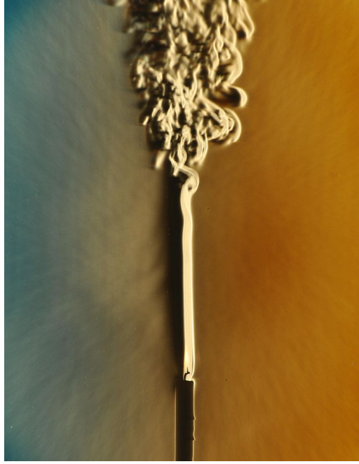
Figure 5.2: The transition of laminar to turbulent flow of a candle flume [15]
