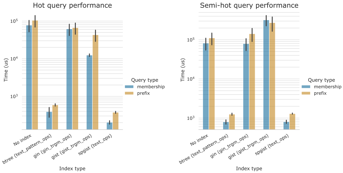
Figure 4.2: Timings of different queries for hot and semi-hot with different index types, error bars are standard error
