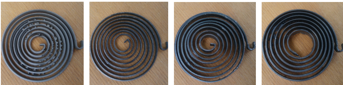
(a) Watercutted 3mm thick spring (b) Lasercutted 2mm thick spring (c) Lasercutted 3mm thick spring (d) Lasercutted 4mm thick spring
