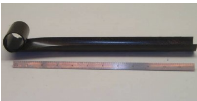
Fig. 12: Neutrally stable composite tape spring by Schultz et al. [38]
