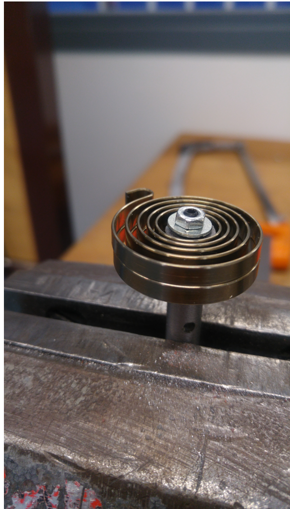
(b) Holding the springs by means of a setscrew, nut and a ring
