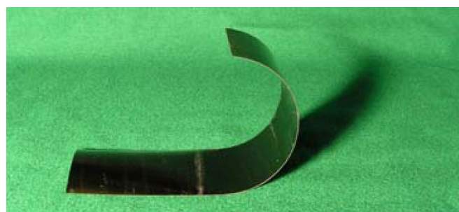
Fig. 16: Neutrally stable tape spring by Murphey and Pellegrino [42]
