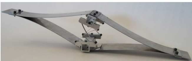
Fig. 23: Zero stiffness compliant joint by Morsch and Herder [49]
