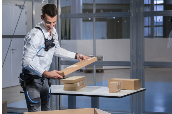
(a) Industrial application Laevo exoskeleton
