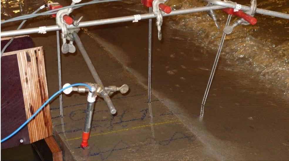
Fig. 3.9.: Three wave gauges and a propeller on the crest.
