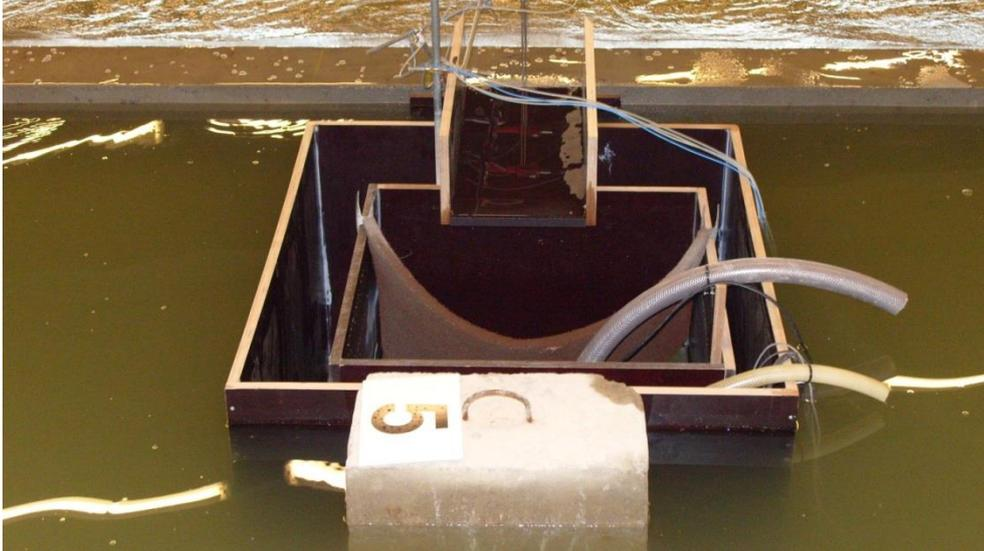
Fig. 3.8.: Overtopping box with pumps and chute.
