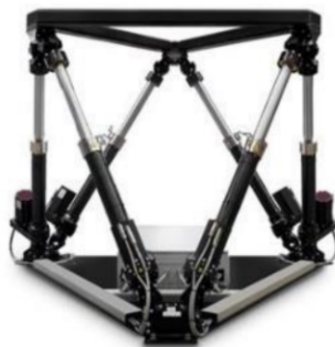
Figure 4.8: A 6 DOF Stewart platform for reproducing the accelerations
