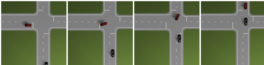
Figure 5.19: Visualization of the scenario with the Ego vehicle taking priority in a left turn and with the other vehicle going straight t = 4 - 7 s
