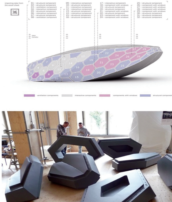
△ Figure 5. Design-to-production of the stage linked the computational design (top left) with numerically controlled production of components (bottom left and right).
