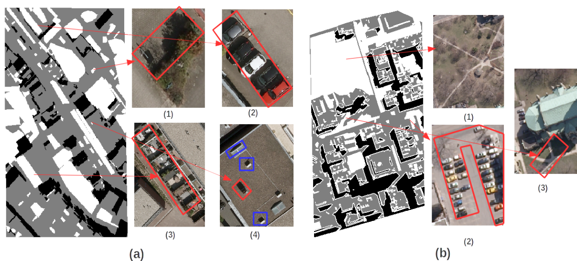
Figure 5. Reference images for Amersfoort (a) and Toronto (b) in the areas indicated in Figure 2b. The black, gray, and white pixels indicate shadow, non-shadow and excluded pixels. In (a), image (1), (2) and (3) show shadow from vegetation, cars and objects in the gardens which are excluded from the reference images, while image (4) shows that if shadows from details on roofs, in the red box, larger than 1m *1m are excluded, and the smaller details in the blue boxes are included in non-shadows. In (b), image (1) and (2) show vegetation and cars are excluded in the reference images, while image (3) shows wrongly labeled areas indicated by reconstructed shadows due to model errors are excluded.
