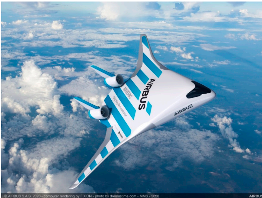
Figure 10-1: Airbus MAVERIC concept of blended wing body (BWB) design, an example of a future aircraft configuration with higher aerodynamic efficiency than conventional tube-and-wings (courtesy Airbus)
